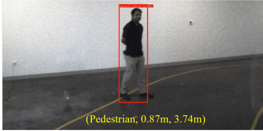
Fig. 3: Detected pedestrian and position estimates.
