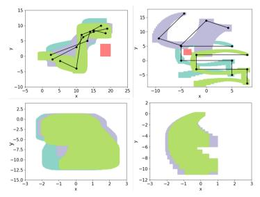
Fig. 1: Reachtubes for three fixed-wing aircrafts (left) and three linear models (right). Real reachtubes (top) vs. the virtual ones saved in *tubecache* (bottom).
