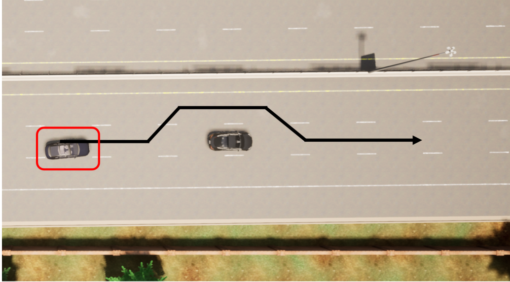
Figure 1.1: This picture shows an example scenario verification problem. The ego vehicle (marked by the red box) is trying to overtake the NPC vehicle stopped in the middle of the lane following the plan specified by the black arrow. We want to show the ego car is able to execute the plan without colliding with obstacles. The scenario is rendered in CARLA [78].
