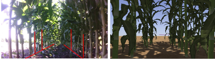
Figure 7.10: Real and simulated camera images for corn row following for agricultural robots.
